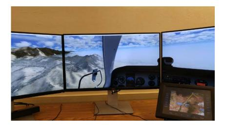
Prepar3D images at 11500ft. The WX image is delayed and shows no cloud cover. The out-the-window shows two distinct layers of clouds.
