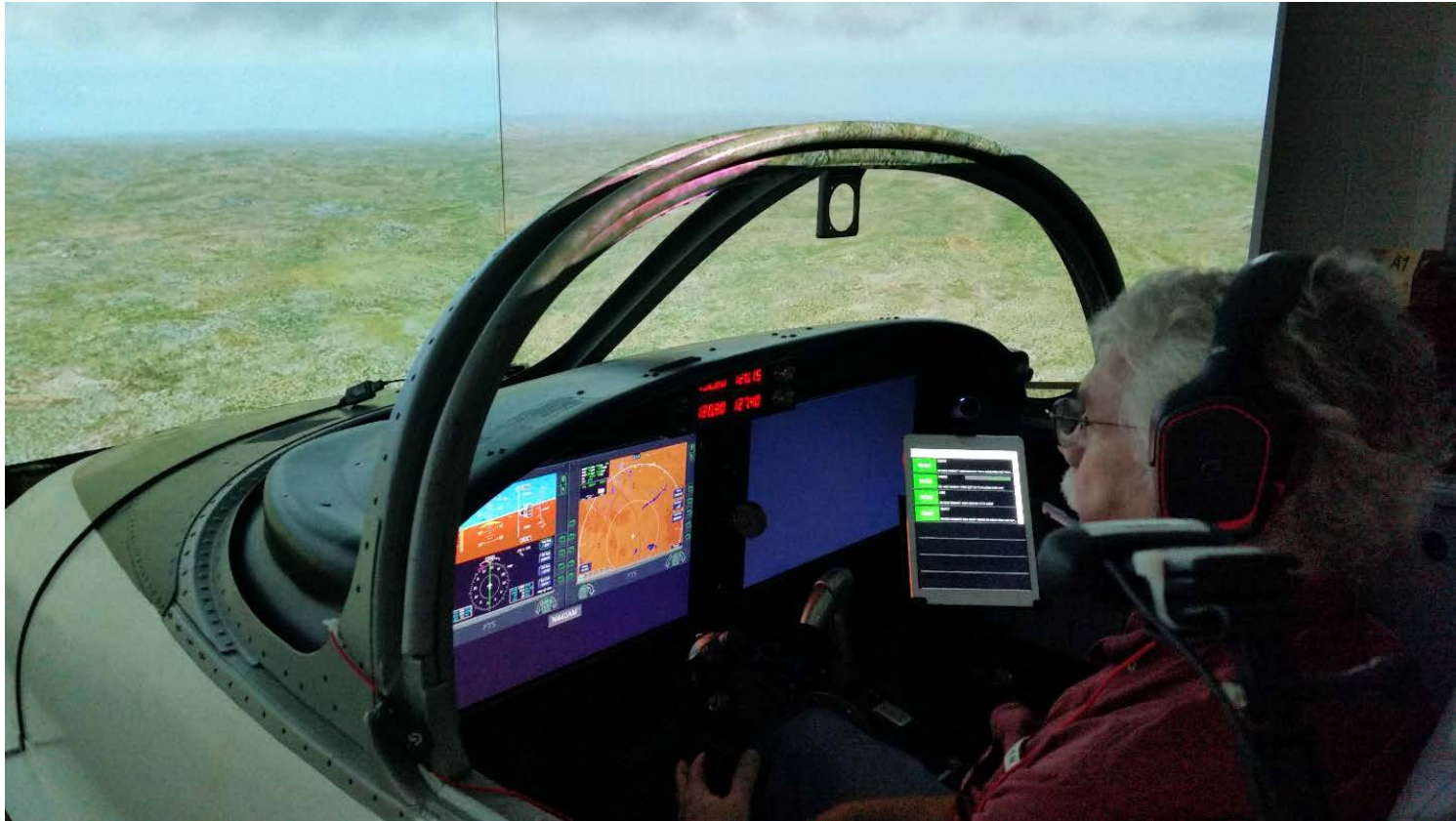
VSCL Flight Training Device, with the mounted Weather Alert Device (iPad)
