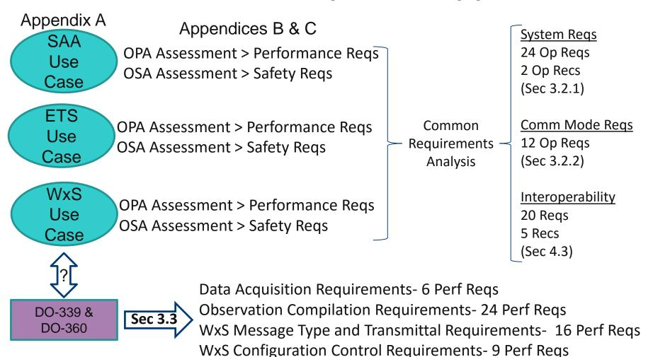
Due to the TORs calling out DO-339 systems and the recommendations from DO-360, Section 3.3 provides requirements for transmission of meteorological and aircraft parameters to enable wake vortex, ATM, and weather applications via the Weather Surveillance (WxS) Service systems.
