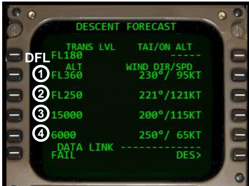
Operational B757 Pegasus FMS (4 DFLs, wind only)
