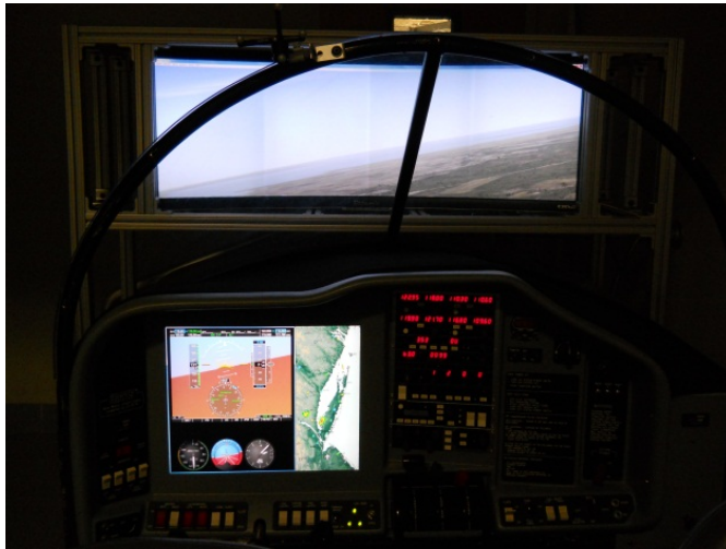
The Micro-jet cockpit simulator (Cessna 172)
