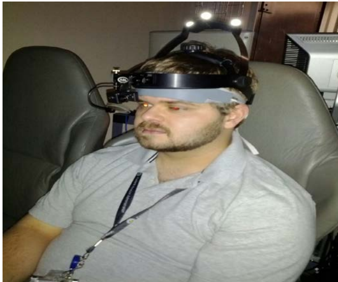
Eye tracker and functional near-infrared (fNIR) systems
