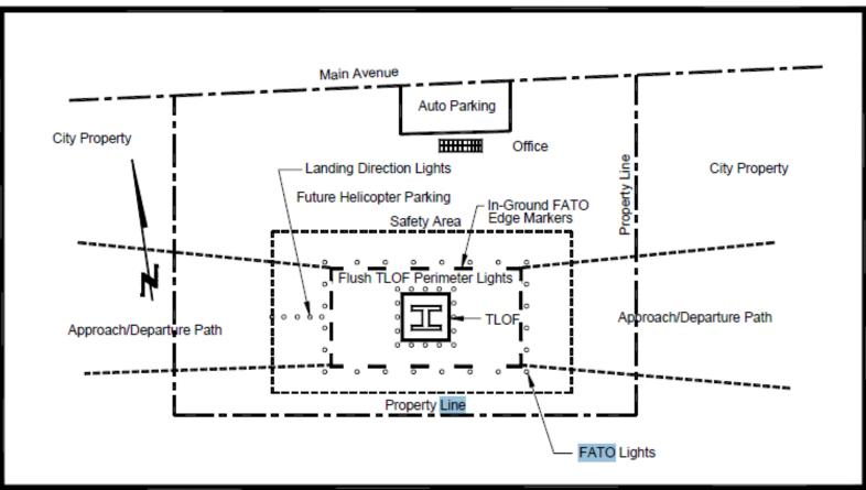
Note: Layout diagrams should be drawn to scale with key dimensions shown such as TLOF size, FATO size, Safety Area size, distances from safety area perimeter to property edges, etc.
