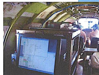
Data Link Test Configuration on LearJet 25 and Display of Weather Information, Atmospheric Data & Traffic
