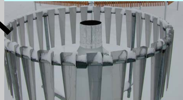
Weighing Snowgauge (GEONOR)
