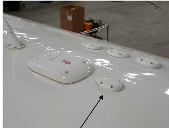
Antenna Aircraft Installation
