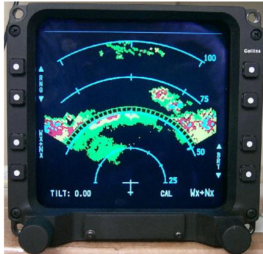
Enhanced Weather Radar: Integrating on-board & uplinked Radar
