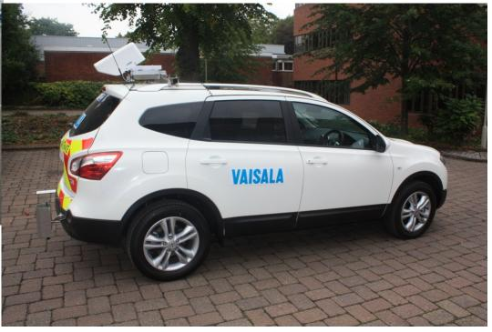
Mobile sensors have enabled Airport users determine what contaminates are on the runway (or other critical areas), reported surface conditions include snow, ice, and water thickness.
