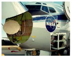
Forward Looking Turbulence Radar
