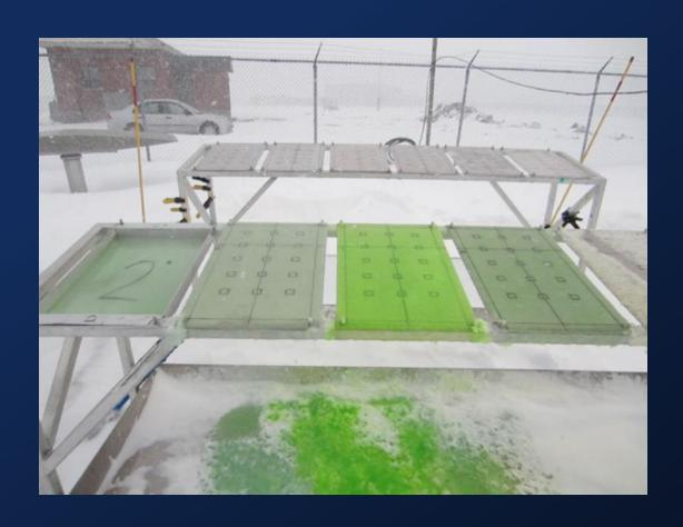
Testing of aircraft anti-icing fluids has traditionally been conducted in an outdoor environment but creates problems
