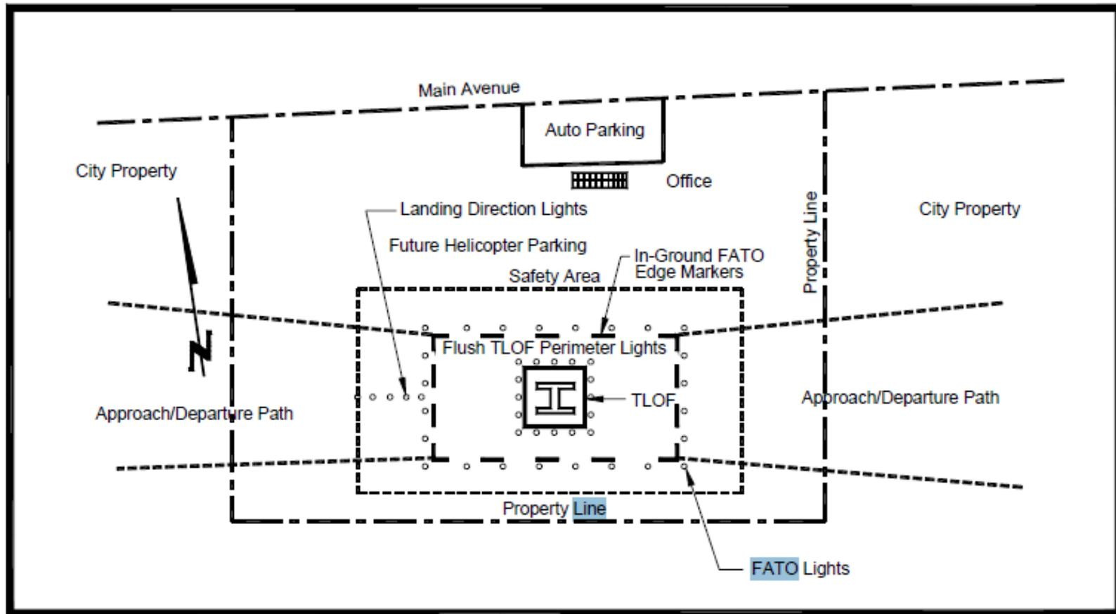
Note: Layout diagrams should be drawn to scale with key dimensions shown such as TLOF size, FATO size, Safety Area size, distances from safety area perimeter to property edges, etc.
